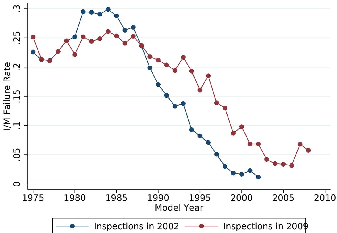
Notes: Lines show the initial failure rate for inspections done in the year 2002 (blue line) and the year 2009 (red line). Vertical axis shows the initial failure rate, while the horizontal axis shows the relevant model year of the tested vehicle.
