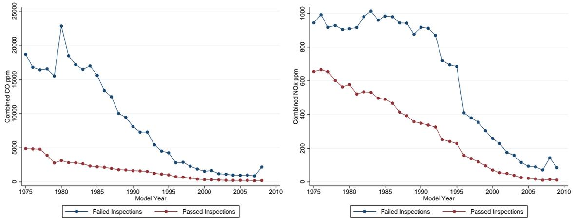
Notes: Graphs show the total combined measured tailpipe emissions at initial test for carbon monoxide (left) and nitrogen oxides (right) from cars that fail (blue line) or pass (red line) initial inspection by model year.
