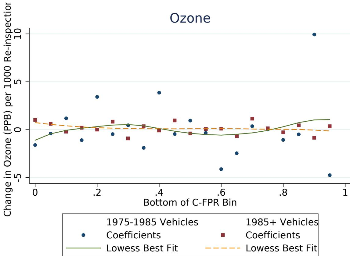
Notes: Graphs show the change in measured county-level air quality for ozone (O3) resulting from an additional nominal 1,000 repairs (as proxied by a successful re-inspection of an initially failed vehicle) done at stations of respective quality as measured across 20 equally-spaced bins covering the full range of our C-FPR measure (see section 4.1). We split results by older (pre-1985) and newer (1985 and onward) model-year vehicles. LOWESS best-fit lines use a bandwidth of  $N * 0.8$ .
